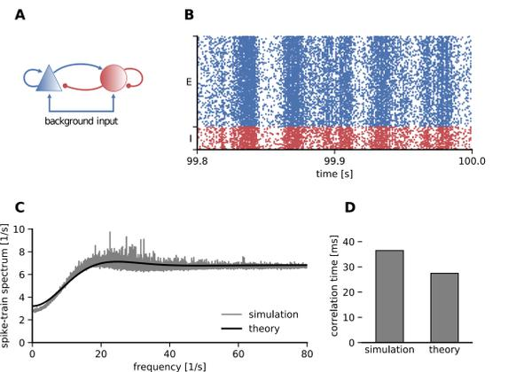
Sketch (A) of a balanced spiking neural network [11] with populations of excitatory (blue) and inhibitory (red) neurons. A raster plot (B) shows asynchronous irregular dynamics with statistically equivalent neurons. The Fourier transform of the autocorrelation function, i.e. the power spectrum, obtained from our theory (C, black line) agrees well with simulations (C, gray line). Accordingly, the predicted intrinsic timescale is also in good agreement (D).
